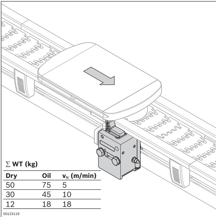
Stop gate for securely stopping a workpiece pallet
