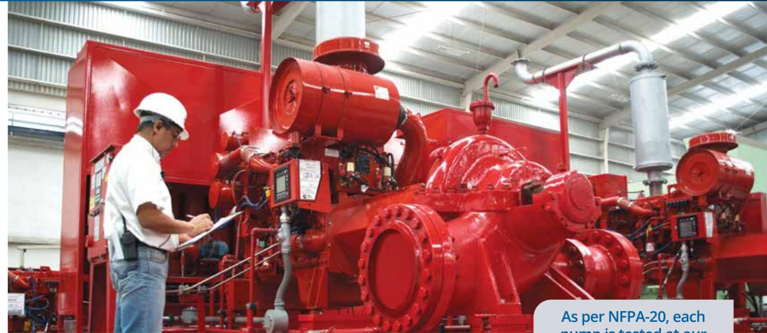
As per NFPA-20, each pump is tested at our manufacturing facilities to provide detailed performance data and to demonstrate its compliance with the required specifications.
