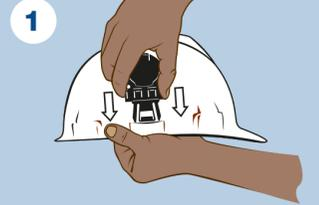
1 Attach adapters to each side of the hard hat by sliding them into the slots.
