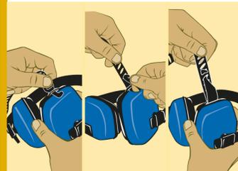
Attach headband strap to the slot in upper part of the earcup when worn behind-the-head or under-the-chin.
