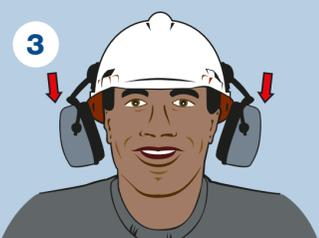
3 Place the hard hat on the head and adjust the earmuffs by sliding the cups up and down.
