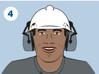
4 Ensure that the earmuff is firmly attached by lifting the arm up and down.
