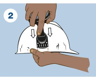
2 Attach each earmuff into its adapter by sliding the earmuff housing down into the adapter,
